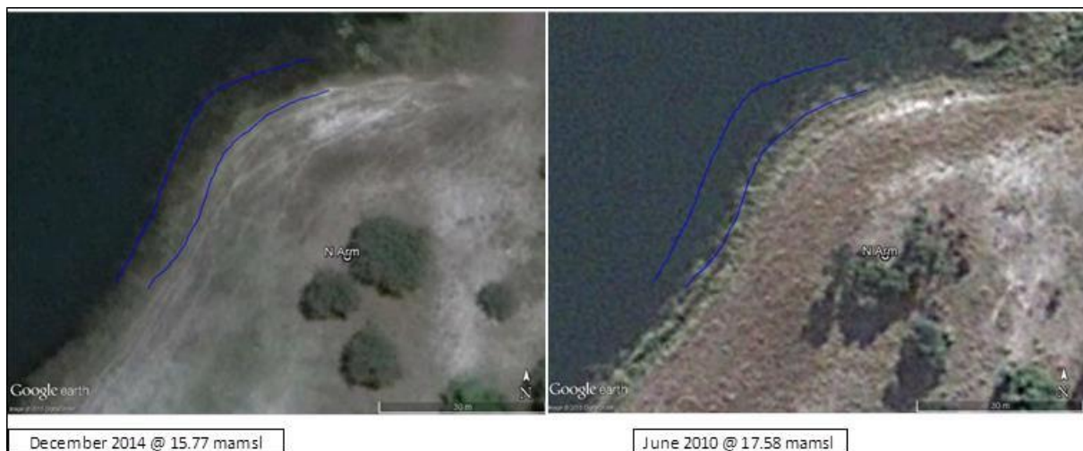
Figure 4.7 Analysis of historic satellite data (Google Earth ©) showed that the emergent macrophyte zone can shift, up to 1.81 m in 4 years i.e. an average rate of decline of 0.36 m/year
