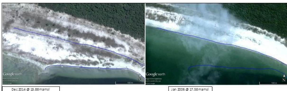
Figure 4.3 Analysis of historic satellite data (Google Earth ©) showed that the emergent macrophyte zone did not shift, although there was an average rate of water level decline of 0.2 m/year
